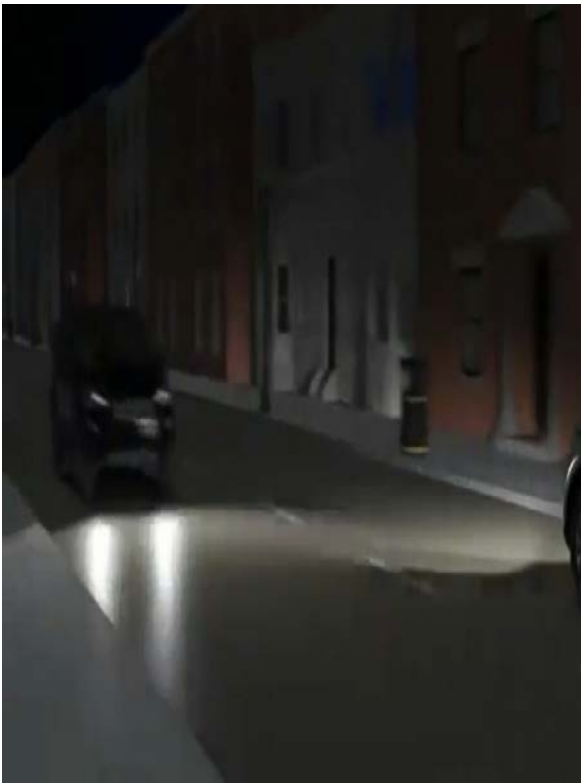
Fig.4: Low beam is activated when there is vehicle approaching from the opposite side
